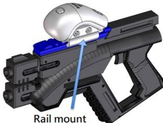
*Figure: Toy like gun with VIVE Wrist Tracker and rail mount-type mounting base*
