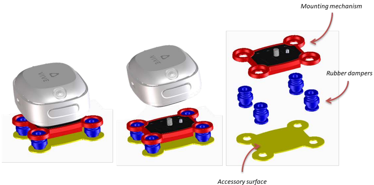
Fig. 9: Attaching a damping mechanism to the VIVE Ultimate Tracker
