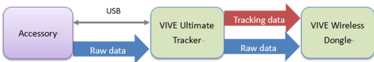
Fig. 2: Wirelessly transmit raw data via USB-C to the VIVE Wireless Dongle connected to a PC or HMD
