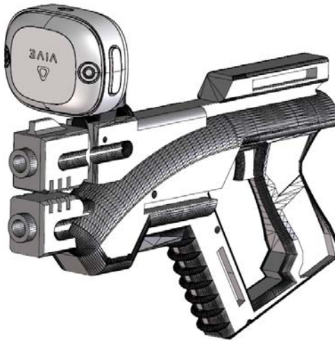
Fig. 10: Mounting the VIVE Ultimate Tracker on a gun accessory
